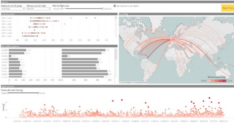
VIEWS is a tool for operational planning, integrating volcano/fire ash/dust storm forecasts updated every 15min with real time data from the VAACs, airlines and engine Original Equipment Manufacturers
